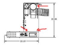
2) Install customer provided PVC 3" to 4" adapter (shown below) to flex tube and secure using provided clamp
