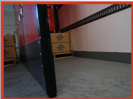
Rear panel offered with a reinforced heavy-duty HMW abrasion plate.
