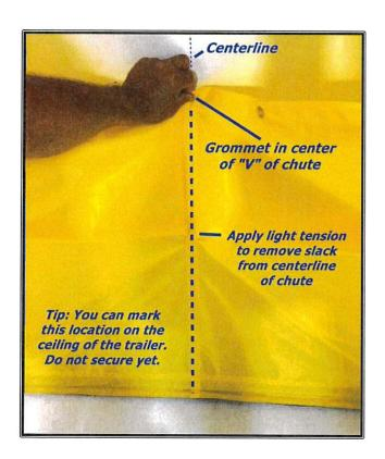
7) On the ceiling centerline, measure 5" towards the front of the trailer (towards the evaporator) and mark the location. Permanently secure the center grommet to the ceiling.
