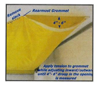
9) <u>Install remaining grommets</u>: Secure the remaining grommets between the center and ends of the "V" of the header.
