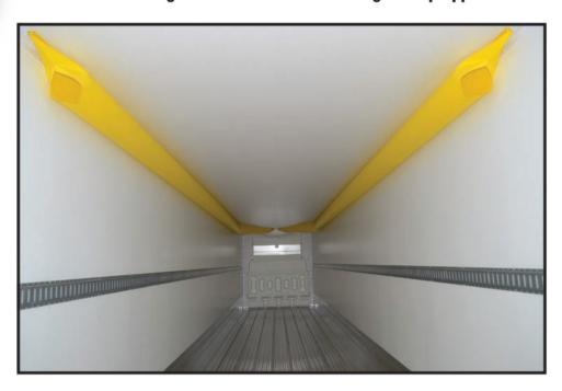
The Tube Chute was designed to provide uniform temperature throughout the entire trailer by using an adapter and chutes that move the air flow from the reefer unit to the rear of the trailer.
