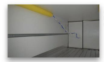
Chute moves air to the back of the trailer reducing reefer run time
